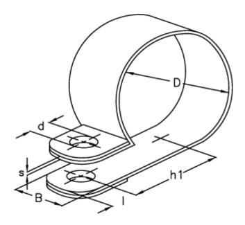
$\begin{array}{ll} d & = 8.4 \\ \text{Diameter D} = 38 \\ \text{h1} & = 31.5 \\ \text{I} & = 8.5 \\ \text{s} & = 0.8 \\ \text{Width B} & = 20 \\ \end{array}$
